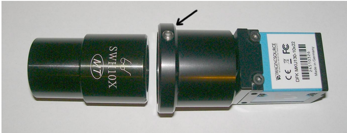
Fig. 2. Camera with attached camera tube and included eyepiece. Arrow: Allen head screw to tighten and loosen the eyepiece.
