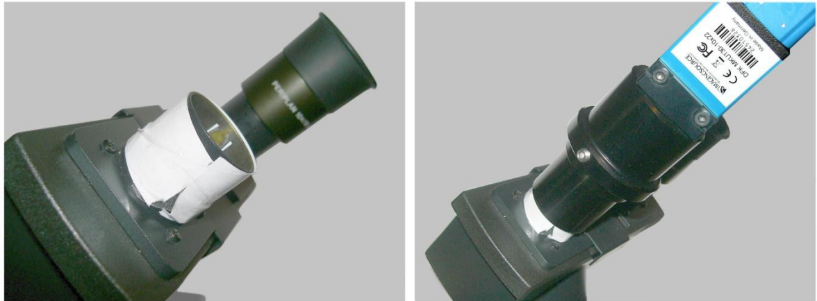
Fig. 3. Use on a tube for eyepieces with a small standard diameter (23.2 mm). The eyepiece head encircled with a paper cuff (left). Camera tube placed on the eyepiece head while using the original microscope eyepiece (shown in the background right).
